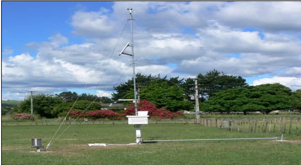
Automated Weather Station for 5 remote outer islands
