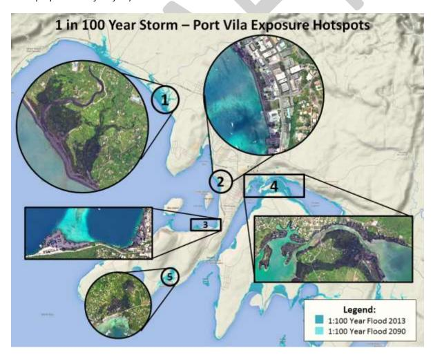
Figure 17: LiDAR modelling of 1:100 year coastal flooding (NAB 2014)
