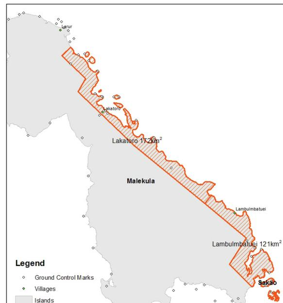
**Figure 2:** Maps showing extent of LiDAR capture in Vanuatu. The orange areas were captured using the topographic (land height) sensor and the blue areas used the bathymetric (seafloor depth) sensor.
