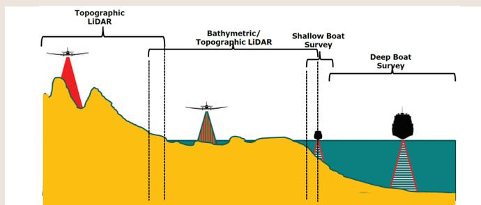
**Figure 5:** Diagram of technologies used to obtain elevation data.
